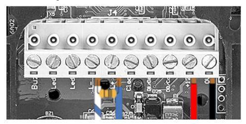
It is important to note that a terminator resistor (typically  $120\Omega$ ) should be installed in parallel across the data leads of the keypad (L- and L+) if this is connection terminates the network. This terminator resistor should be as close to the terminal block as possible. If possible the terminating resistor should be protected by heat shrink.
