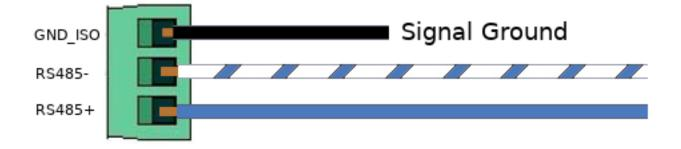
There is no need to install a terminating resistor at the RGO. If the RGO is the terminal connection then a built-in terminating resistor  $(120\Omega)$  can be enabled in software.
